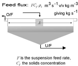
Fig. 6.9 Flux ( $\text{kg s}^{-1}$  of solids) fed to the thickener
