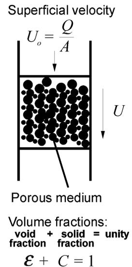
Fig. 6.1 Illustration of porous medium - including settling suspension
