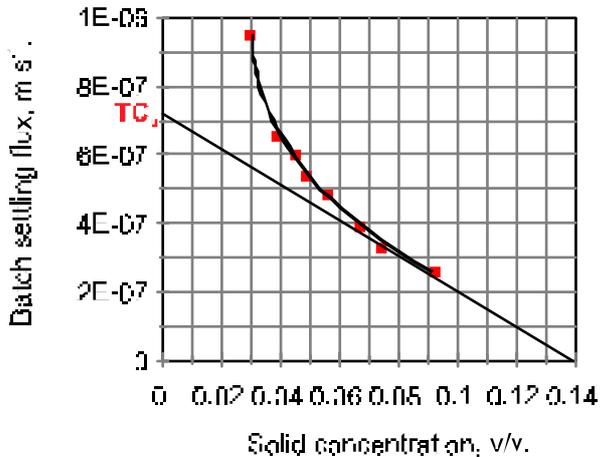
Now a flux balance on a thickener provides the following result:
